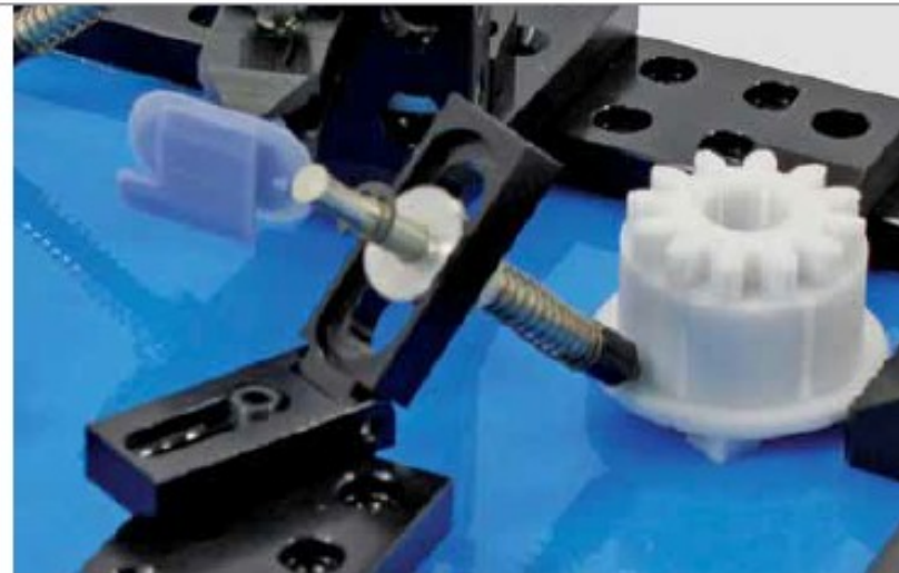
A push rod enables positioning from an angle
