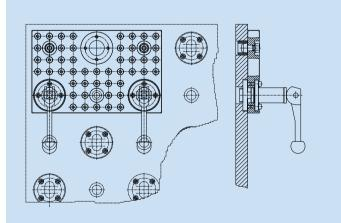
This type of sandwich plate is suitable for example for mounting PPS adapter plates
